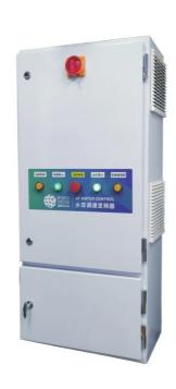
**AF WATER CONTROL** Pump speed controller can protect the circulation pump. When the inlet or outlet water pressure is not enough or the water flow is insufficient, it will automatically cut off the power supply to prevent the circulation pump from idling, protect the pump, and also extend the working life of the pump.
